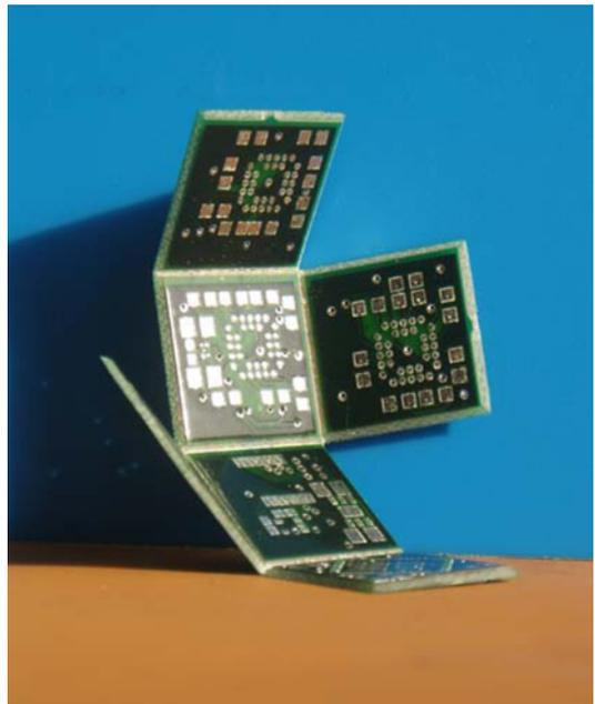
Fig. 1. First prototype of the highly miniaturized inertial measurement unit mCube, unpopulated and half folded.
