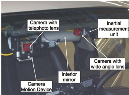
Fig. 3. Camera motion device and inertial measurement unit mounted in a test vehicle. The rigidly mounted camera gives an overview of the environment and detects points of interest for the pivotable camera with telephoto lens.
