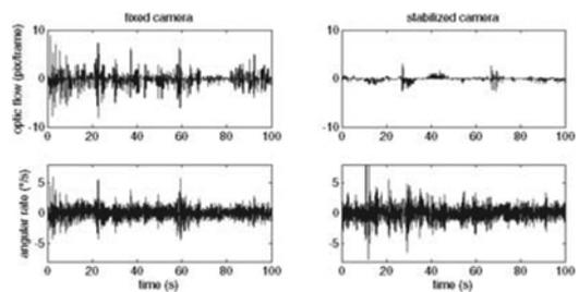
Fig. 4. Optic flow and angular rates (pitch) during test drives with target fixation 40m ahead for the stabilized camera (right) and a reference drive with actuators switched off (left).
